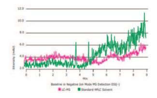
LC-MS grade solvents such as PurSolv Ultra provide consistently low and stable baselines, ensuring higher sensitivity and reliability compared to standard grades.
